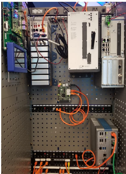
This IIC Testbed Demonstrator in Austin, Texas, shows multi-vendor products that were "plug-and-play" tested for interoperability of TSN synchronization. At center is a Hilscher netX chip-based board.
