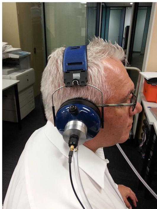
**Fig. 14** Pneumatic driver constructed using earmuffs with attached tubing and low-frequency microphone [64]
