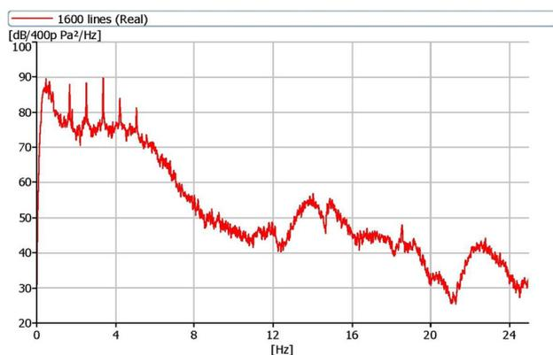
**Fig. 3** Measured infrasound power spectral density spectrum (1600 lines 0–25 Hz) showing a fundamental blade pass frequency of 0.85 Hz and harmonics recorded inside the bedroom of a residence located 1.6 km from Cape Bridgewater Wind Farm, Victoria [32]
