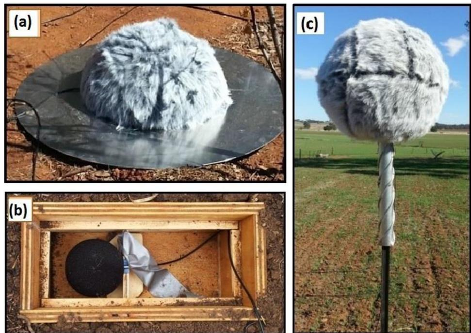
**Fig. 2** a Hemispherical windshield, b submerged box windshield and c spherical windshield [30]
