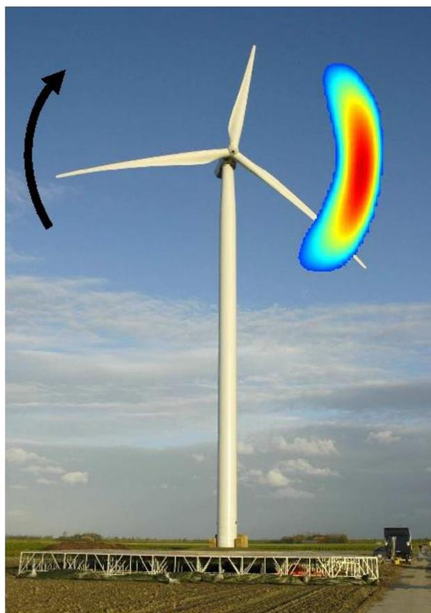
**Fig. 1** Test set-up with GE 2.3 MW turbine with 94 m diameter rotor and microphone array platform. The noise sources in the rotor plane (averaged over several rotations) are projected on the picture [28]
