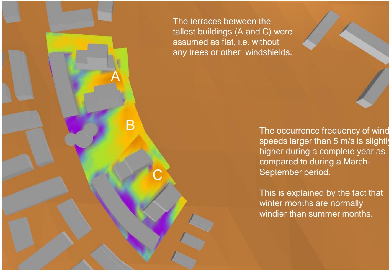
Percentage of time (%) when the perceived wind speed exceeds 5 m/s
