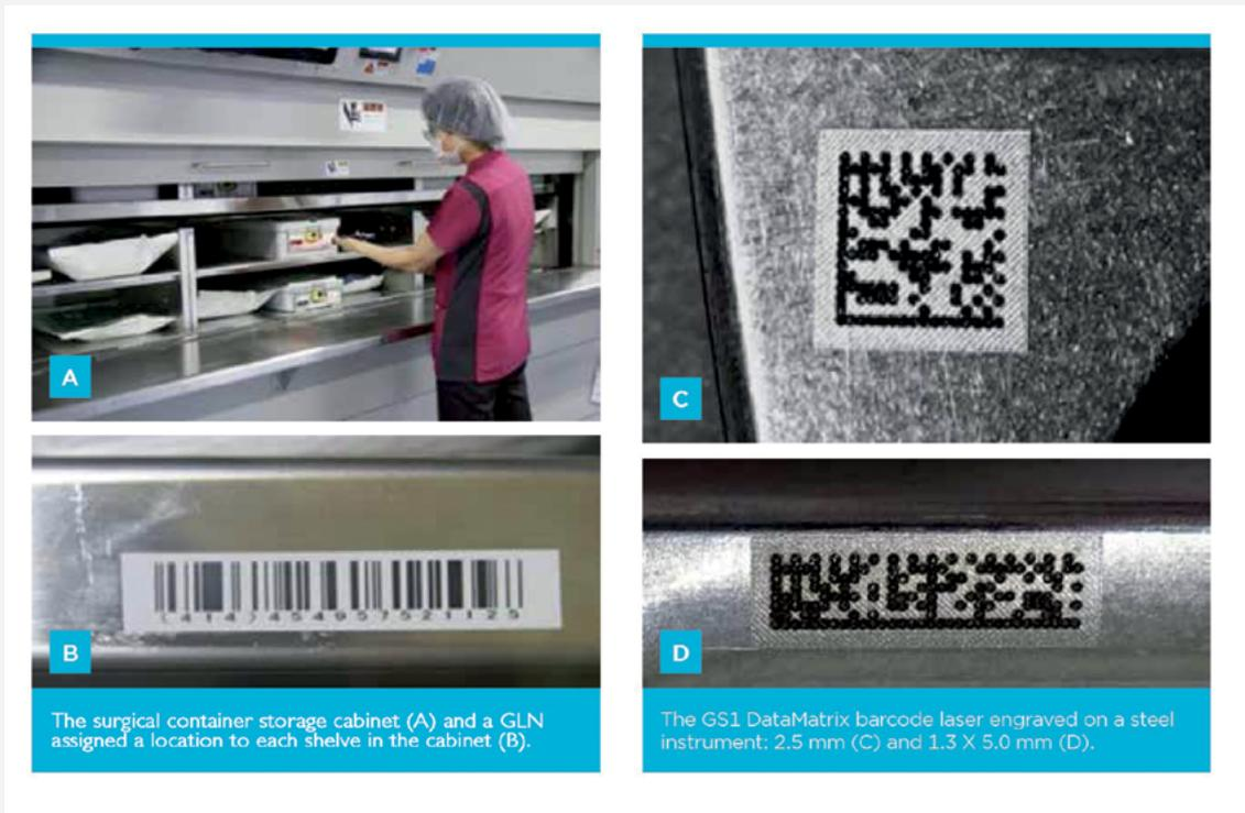
The hospital's surgical container storage cabinet (A) and a GLN assigned a location to each shelf in the cabinet (B). The GS1 DataMatrix barcode laser engraved on a steel instrument: 2.5 mm X 2.5 mm (C) and 1.3 X 5.0 mm (D).
